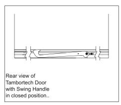
All shelving MUST be set back a minimum of 50 mm from Gable/Blade front edge for the Swing Handle to function properly.
